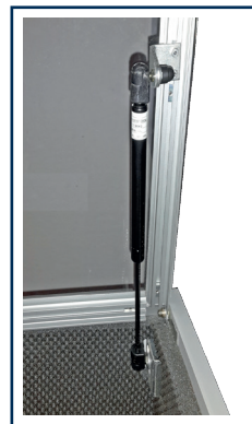
Gas-filled shock absorber
