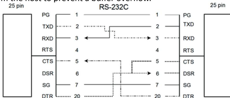
**Note:** Printer DTR may be connected to host DSR + CTS or only to host DSR and a bridge between RTS and CTS
