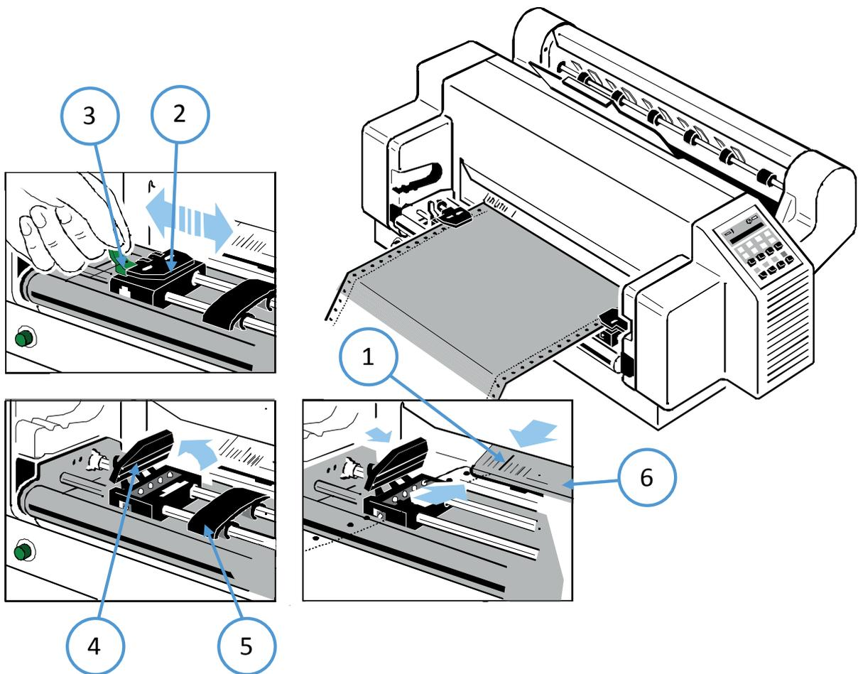
**Attention:** Only move on tractor base (2) not on flaps (4) iehen (danger of breakage)
