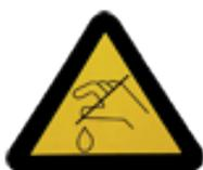
This symbol is visible when the top cover has been opened. It indicates that the print head is extremely hot after leing periods of printing.
