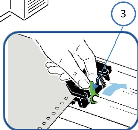
**Note:** The paper should be inserted taut, but not overstretched and the transport pins must be in the middle of the transport holes!
