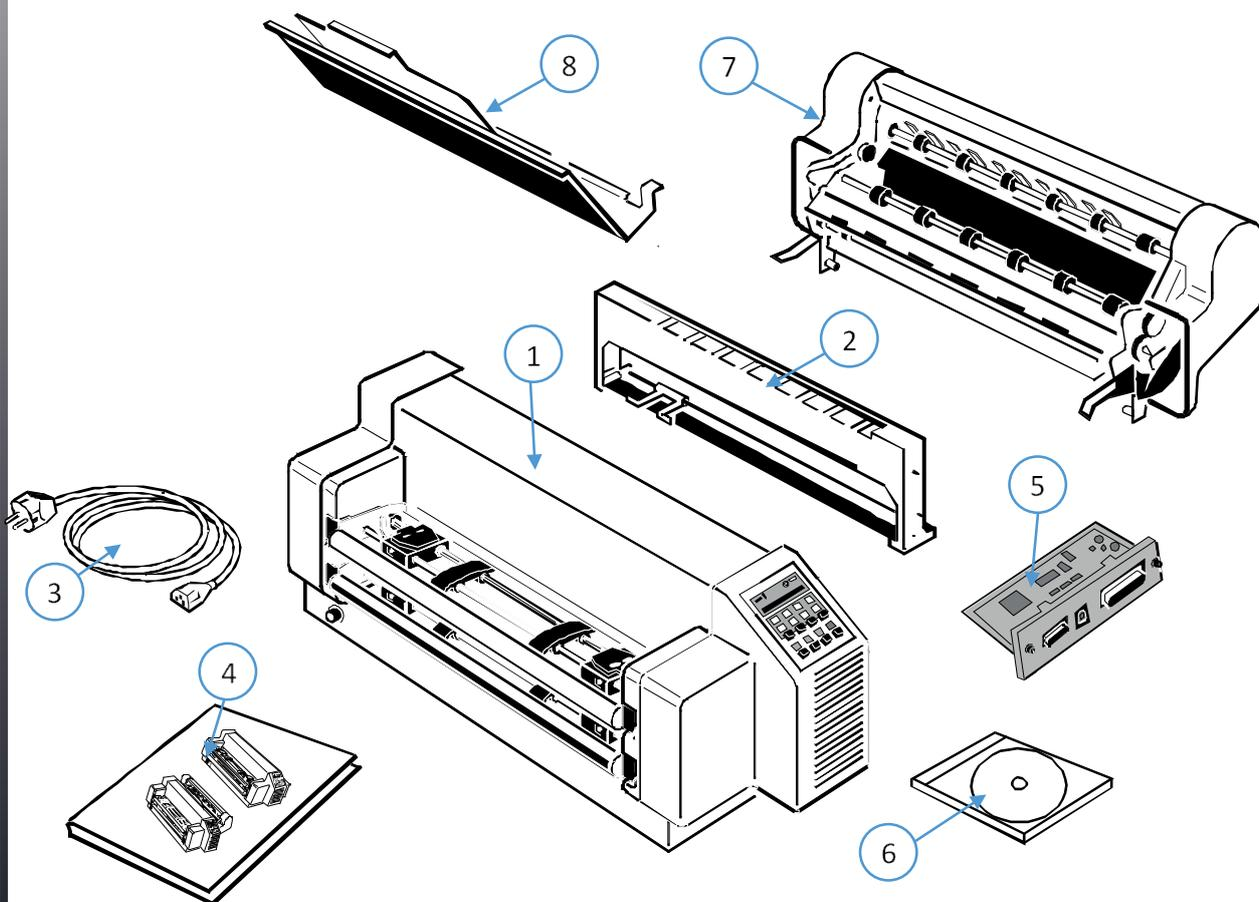
An interface module (5), also called “Personality Module” or briefly “PM”, is in a separate packing and must be ordered separately.
