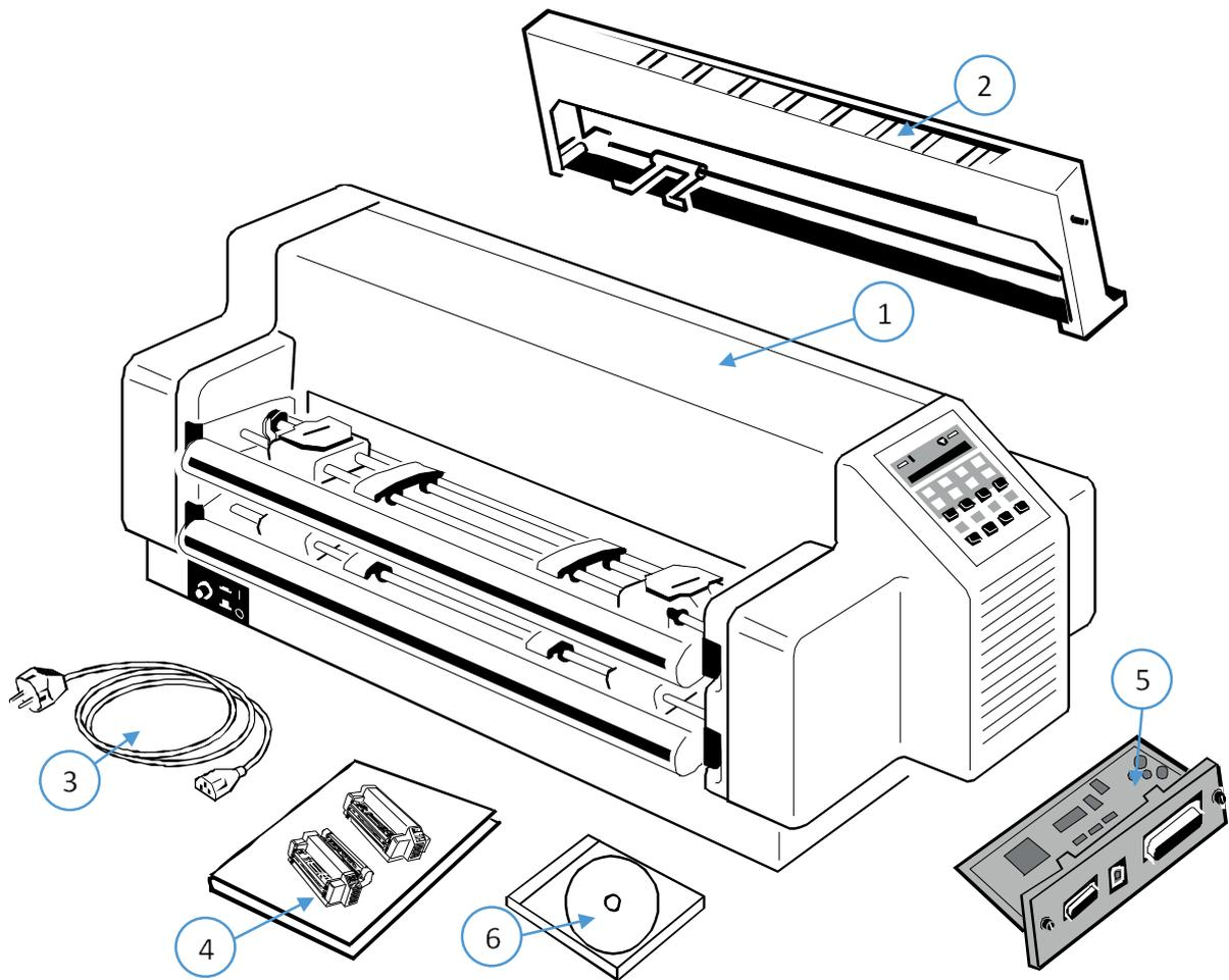
An interface module (5), also called “Personality Module” or briefly “PM”, is in a separate packing and must be ordered separately.
