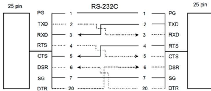
For local connections **RTS** with **CTS** can be connected and likewise **DTR** with **DSR**
