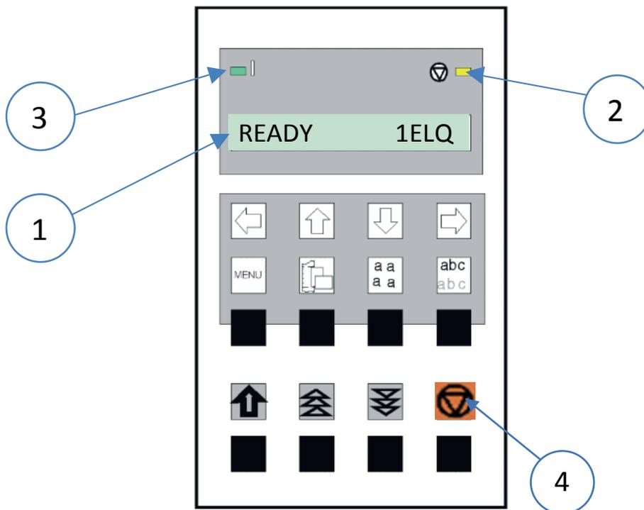
The 16-character Liquid Crystal Display (LCD) (1) indicates the current status of the printer. If an error occurs (e.g. COVER OPEN), the resulting error message overrides any other displayed message. When the error condition no longer exists, the original status information appears on the display.
