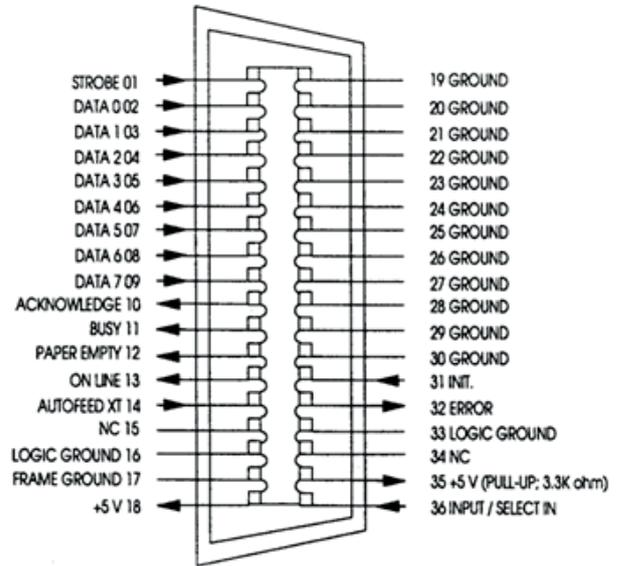
The ACKN pulse informs the host that the data has been received and that the printer is ready to receive new data. If the interface buffer is full except for the last character the BUSY is not reset in order to stop the data transfer from the host. The BUSY signal is only reset if space is available in the interface buffer for a minimum of 512 characters.
