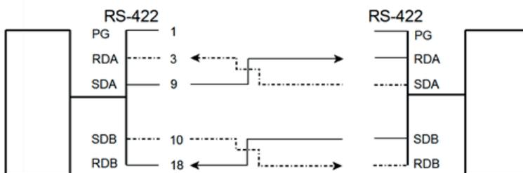
**Note:** Protective ground (PG) connected either to host **or** printer
