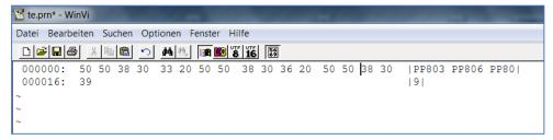
Additionally the file STGCHG.out can be transferred to the printer, in order to examine the correct print. Before it must be paid attention to the correct menu setup of the printer regarding emulation etc.
