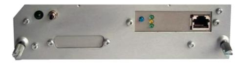
For downloading a StringChange – definition file depress and hold the push button while the printer is powered on. The green LED is on until the download process begins and off after termination. While download of larger files the LED is blinking. The description for the Ethernet interface is available in a separate documentation.
