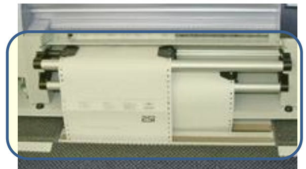
Movable printer tray for easy ribbon installation
