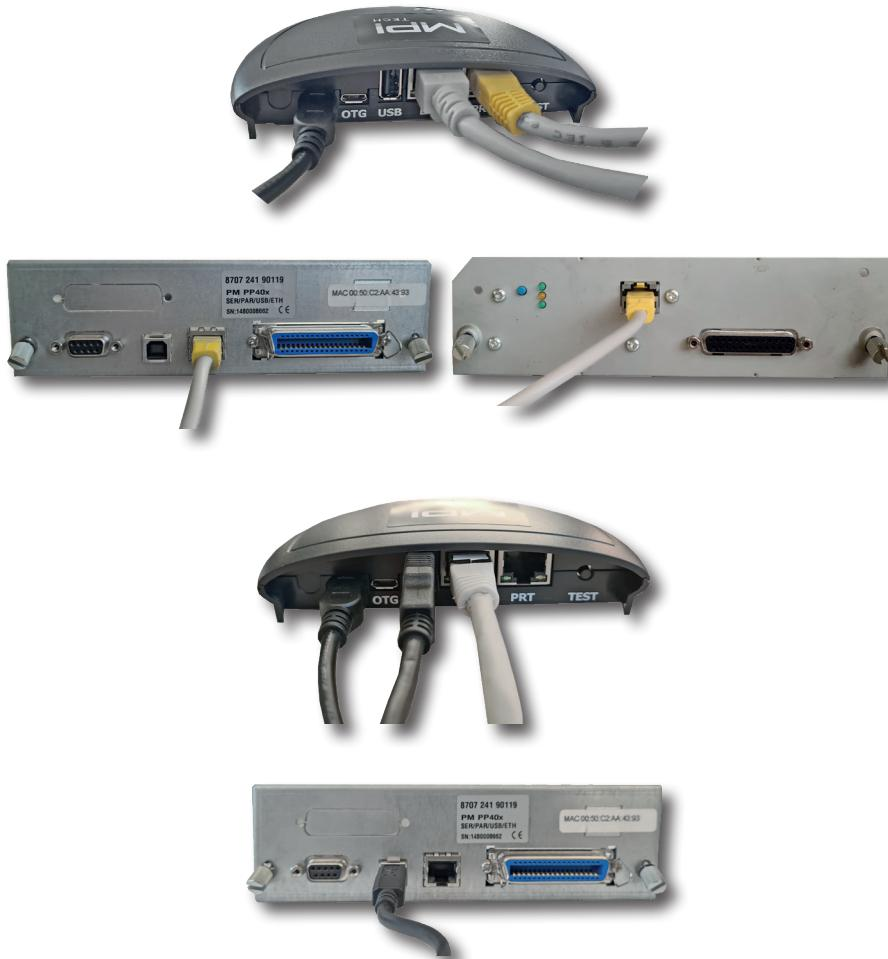
IPDS LAN connection for PSI printers of the PP 40x and PP 80x families with MPI EasyCom 5 print servers. This hardware unit transforms the printers into IPDS network printers. The EasyCom 5 IPDS PrintServer can be connected directly to the USB port of PP 40x printers or via the existing network connection „RJ45“ of the printer interface. With PP 80x only via „RJ45“ connection.
