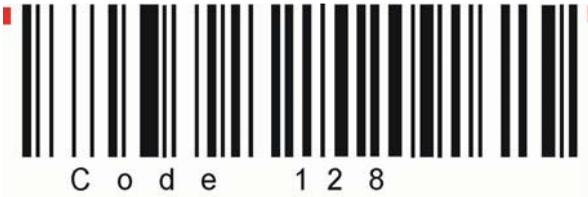
**Bar Code Example for Code 128 using FNC1 = Coding ] C 1**
